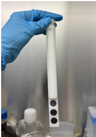
Figure S1. Stainless steel coupons used in biofilm experiments.
